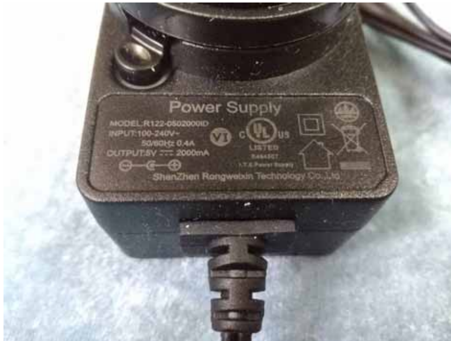
Photo 15 Marking of switching power supply
