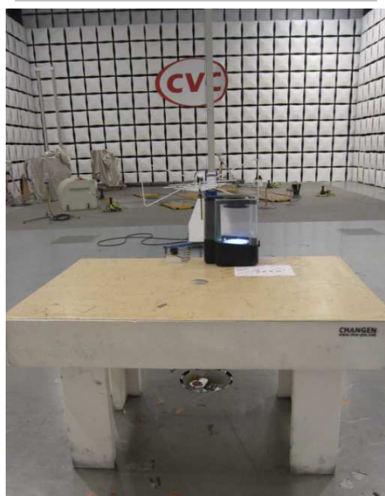
Radiated Disturbance (30MHz~1000MHz)
