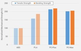
Tested with 3D printed specimens (100% infill)
