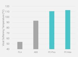
\*Tests performed with 3D printed specimens (100% infill, standard Vicat conditions)
